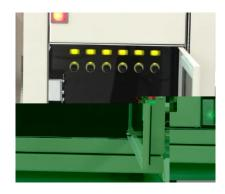
The intelligent cabinet does not allow to take any keys, just those, which the person is entitled for in the given time. Green led indicates the keys which can be taken, red means locked, not authorized keys By default, the cabinet identifies the person and the key. Booking, finding, banning keys are available services, just like setting alarm on not returned keys.
