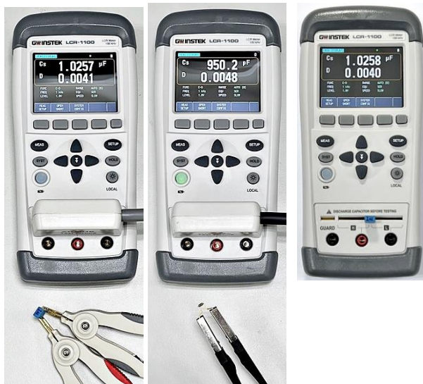
Figure Test results for capacitors
