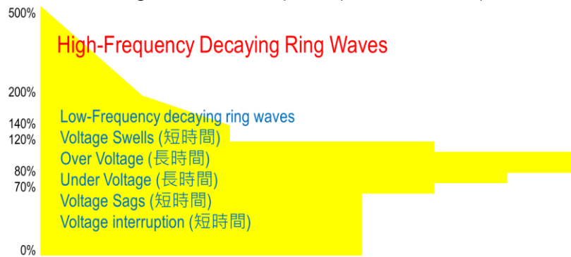
Figure 3 Schematic diagram of power quality issues of no interruption in function region Note 5: TVSS Transient Voltage Surge Suppressor
