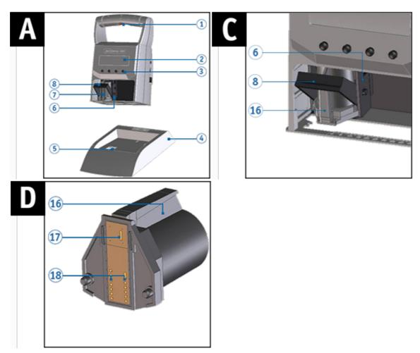
In rare cases, impurities on the contacts of the print cartridge <sup>18</sup> can cause incorrect printing results.
