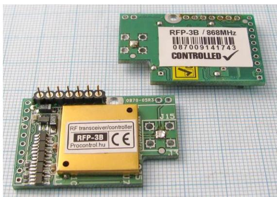
RFP-3 is a hybrid data radio module built with nRF true single chip system: integrated radio frequency transceiver with embedded microcontroller and a 4 input (10bit 80ksps) ADC converter, antenna filter and adapter system for connecting an 50 Ohm antenna, 50 Ohm SMA antenna connection prepared.
